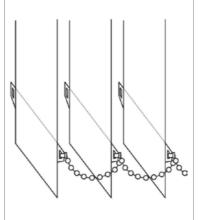
Tip: Lifting the hook on the chain, over & down onto the weight tends to prevent potential damage.
