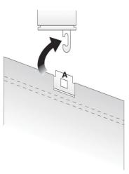
2. Face Fixing Lightly screw short screws into place. Position brackets approx 5cm from the ends of the headrail. Mark holes A and screw brackets into place.
